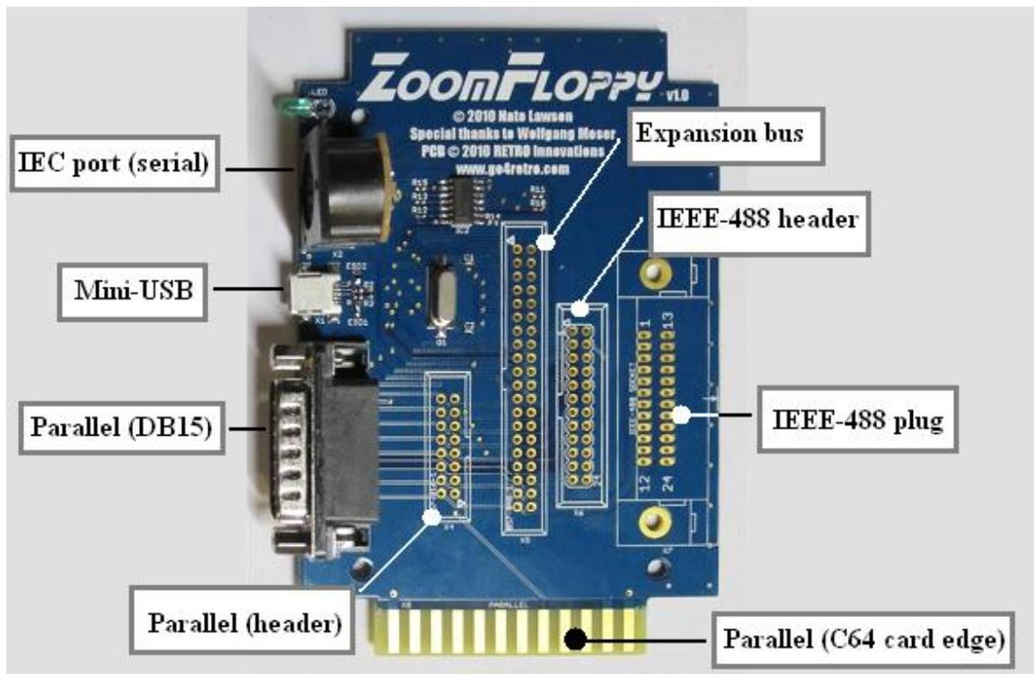
At a minimum, the ZoomFloppy must be connected to one or more floppy drives via the IEC serial port (6-pin DIN) and to a computer via USB. It is powered over USB, so no external supply is needed. This configuration gives basic access to read and write disks. OpenCBM provides some faster serial transfer routines and defaults to auto-selecting the best one for your configuration.
